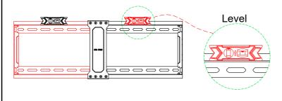
7-2 Use bolt holes at same level, and pull bracket upward to reduce the gap between the hole and bolt, then fasten them finally.
