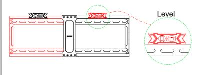
5-2 Use bolt holes at same level, and pull bracket upward to reduce the gap between the hole and bolt, then fasten them finally.
