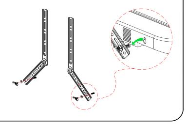
Case 6 The TV VASE hole does not match the soundbar hole or does not match the screw
